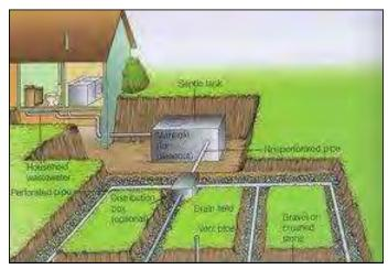
A Septic System consists of various components including: Septic Tank, Inlet wastewater pipe and a Drain field/Soak away. Waste water from the property flows into the Septic Tank directly from the drainage pipes from the sinks and toilets.
