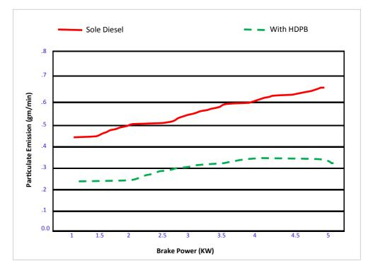
It is seen from the graph the particulate emission is Reduced when diesel blends with Hydra Diesel Power Blast.
