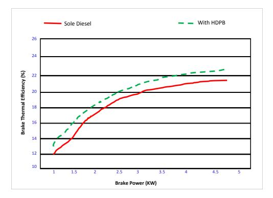
Above graph indicates the variation of Brake Thermal Efficiency with Brake Power of the engine. The Brake Thermal Efficiency at full load condition is increased with the use of HDPB and this is due to full atomization of the fuel.
