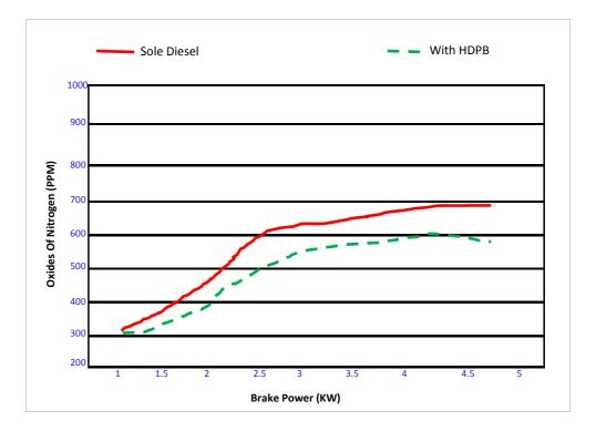
Above graph shows the variation of NOx emission with brake power of the engine. It is seen that for HDPB blend emits lower NOx level compare to standard diesel.
