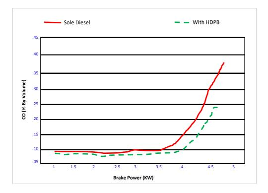
Above graph shows the CO emission with brake power of the engine, the CO level for Hydra Diesel Power blends is less than the sole diesel fuel at full load.
